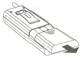
2. Insert 8 alkaline batteries into the battery compartment as shown.
